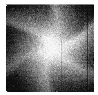
Iris shutter vignetting pattern. This image is produced by dividing a short (1 second) exposure dome flat by a long (30s) exposure dome flat.
