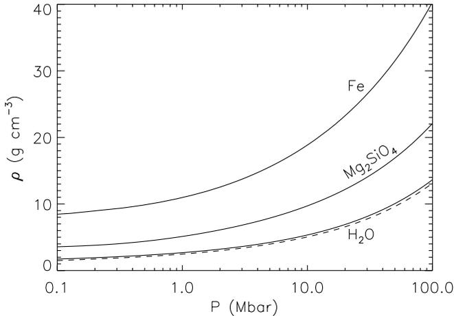
FIG. 1.—Zero-temperature pressure-density relations for iron (Fe), rock ( $\text{Mg}_2\text{SiO}_4$ ), and water ice ( $\text{H}_2\text{O}$ ). For ice, the dashed curve shows our EOS with the thermal correction described in § 4.1.
