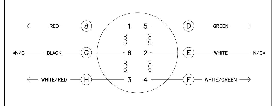
\* = NOT CONNECTED TO DRIVE GROUND. THESE LEADS MUST BE INSULATED AND ISOLATED OR DAMAGE TO DRIVE MAY OCCUR
