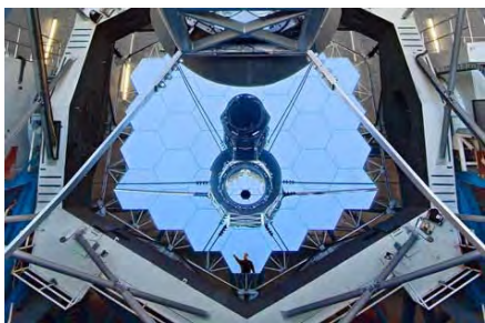
Figure 11. The 36 segments of the Keck II primary mirror.
