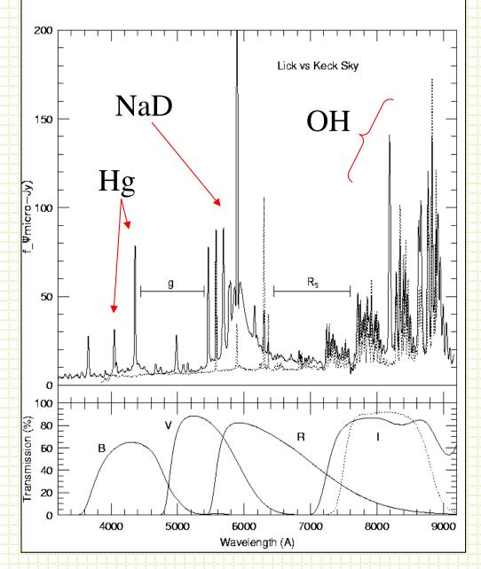
Signal from the sky background is present in every pixel of the aperture. Because each instrument generally has a different pixel scale, the sky brightness is usually tabulated for a site in units of mag/arcsecond<sup>2</sup>.
