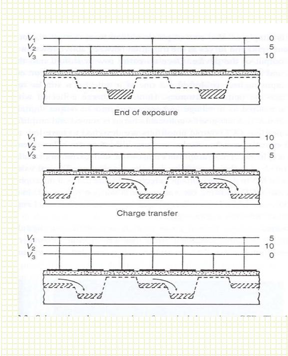
• Example threephase readout to create bucket brigade and move accumulated charge into readout amplifier
