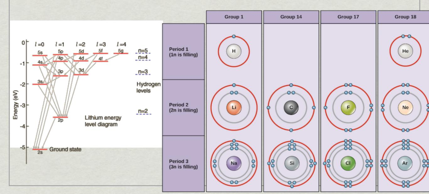
Get energy = absorb a photon, electron moves to a higher energy level Release energy = emit a photon, electron falls to a lower energy level
