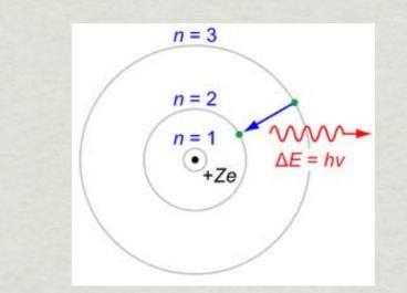
Get energy = absorb a photon, electron moves to a higher energy level Release energy = emit a photon, electron falls to a lower energy level
