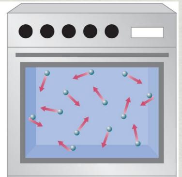
Higher average kinetic energy of a single particle: higher temperature
