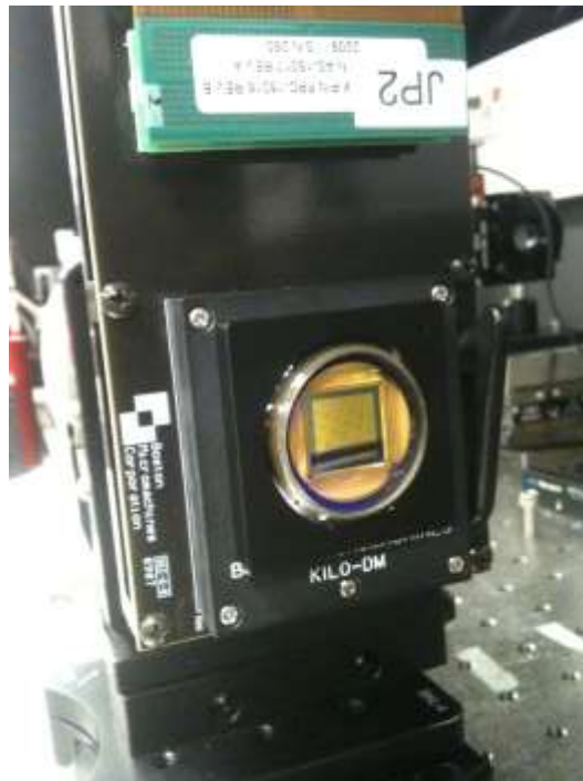
Figure 10. The Boston micromachines Kilo-DM under test at the Laboratory for Adaptive Optics.
