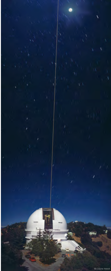
Figure 1. Lick Observatory 3-meter with laser guide star system in operation
