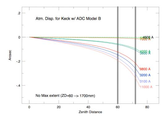
This figure looks similar but not exactly the same as for the sub-aperture model. The difference is almost certainly due to some inaccuracy or round-off in calculating the "best" prism separation. Relative to the previous case, the IR is correctly slightly better at the expense of the UV correction.
