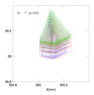
The figure to the right is a typical spot diagram showing ADC-corrected images at all the sample wavelengths. This is at Z=55 and 1400mm separation.
