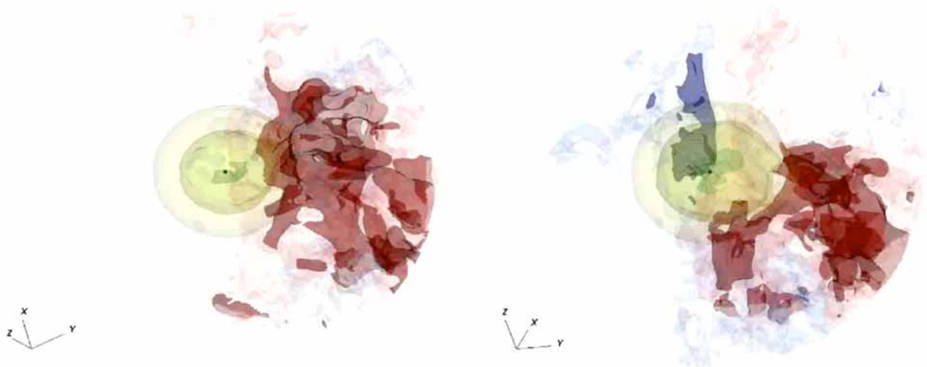
MAESTRO simulations of convection in a non-rotating white dwarf (left) and a 1.5% Kicpation rotating white dwarf (right) preceding a Type Ia supernova. Each simulation uses adaptive mesh refinement with an effective 768^3 zones (6.5 km spatial resolution).
