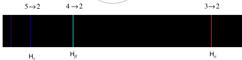
Hydrogen emission line spectrum Balmer series
