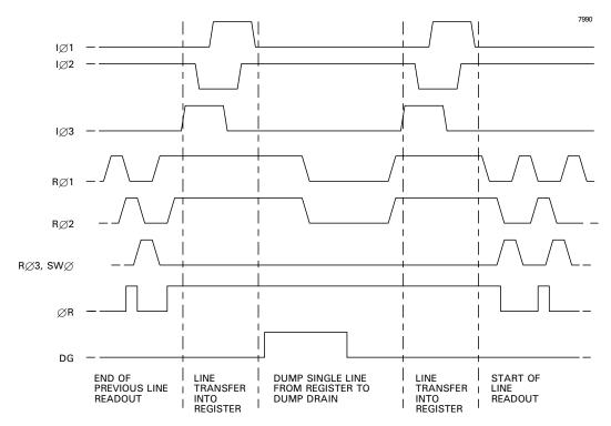
DETAIL OF VERTICAL LINE TRANSFER (Multiple line dump)
