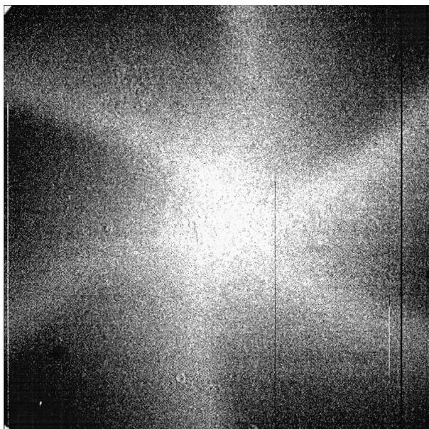
Iris shutter vignetting pattern. This image is produced by dividing a short (1 second) exposure dome flat by a long (30s) exposure dome flat.
