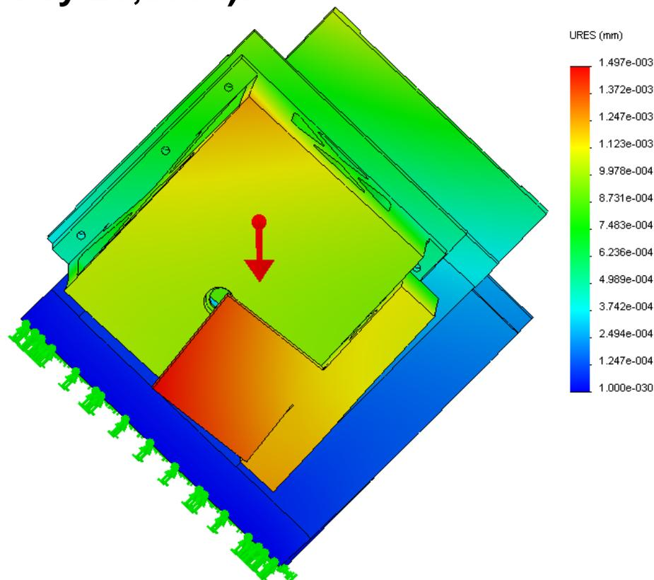
Load: Telescope at 45 Degrees from Zenith (about Z axis)
