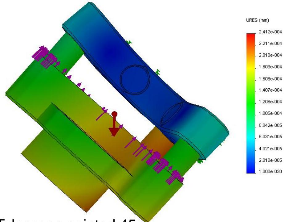
Telescope pointed 45 degrees West (0.24 micron max deflection)
