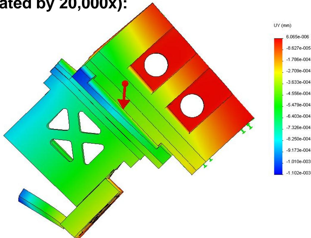
Load: Telescope at +45 Degrees from Zenith (about X axis)
