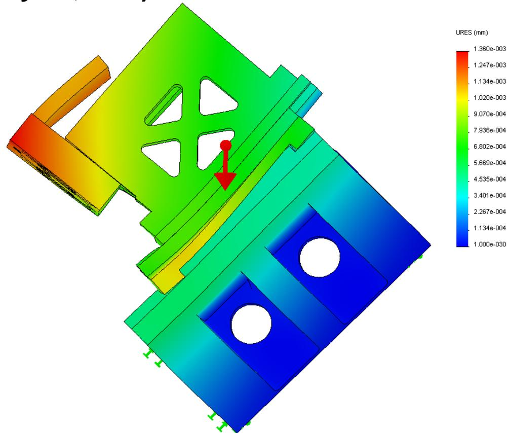
Load: Telescope at -45 Degrees from Zenith (about X axis)
