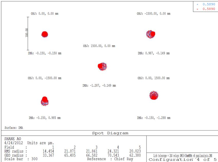
The spot diagram at left shows geometric spots from the center and edges of the primary mirror, as imaged on the lenslet array. The lenslet array pitch is shown on the scale bar. Similar results for 8x8 and 26x16 subapertures.
