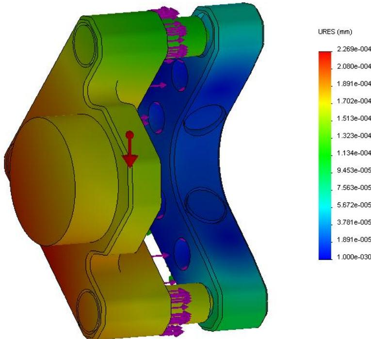
Telescope pointed 45 degrees East (0.23 micron max deflection)
