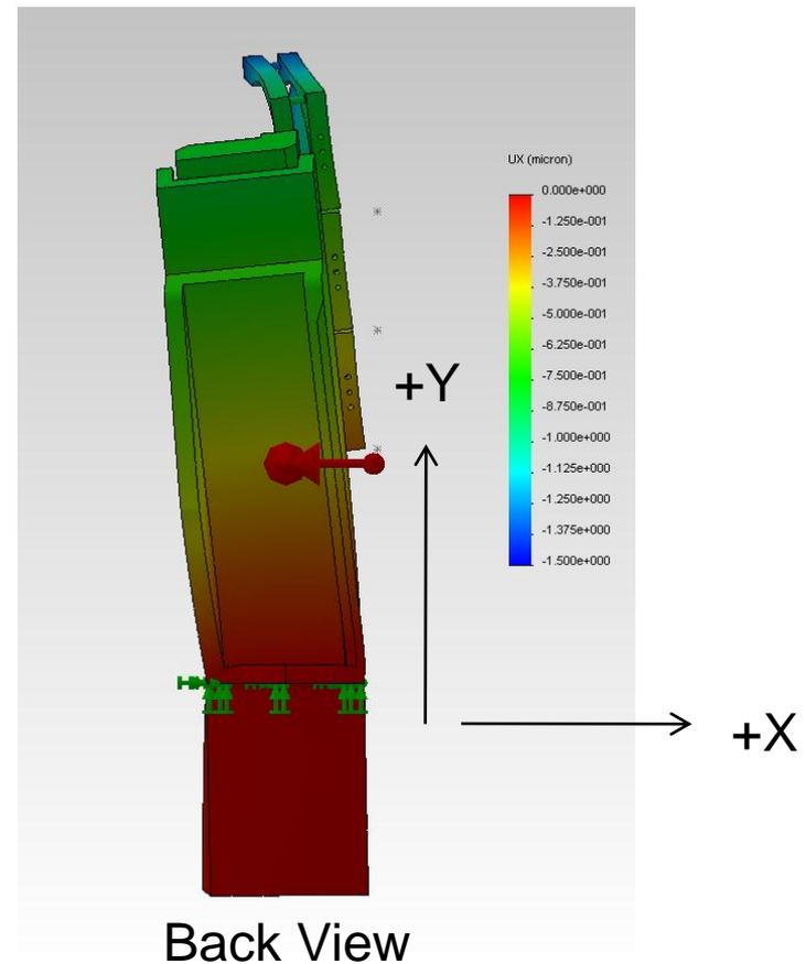
Case A: Telescope pointing straight up "0 degrees"
