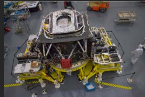
spacecraft bus at NGAS (the hot side of JWST!)
