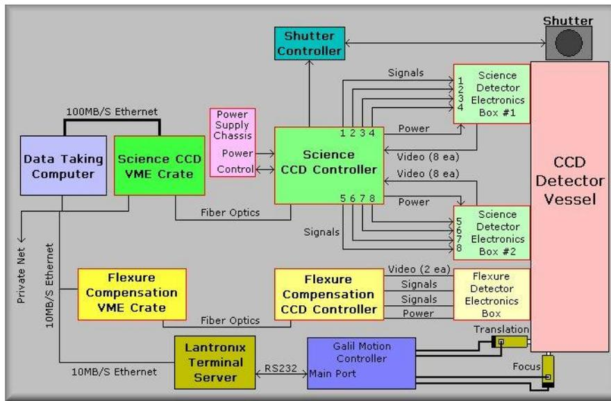
**Figure 1.** Block diagram of the CCD imaging systems within DEIMOS
