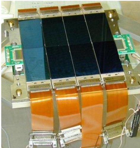
**Figure 4.** Science Mosaic with FC CCDs located on the left and right sides
