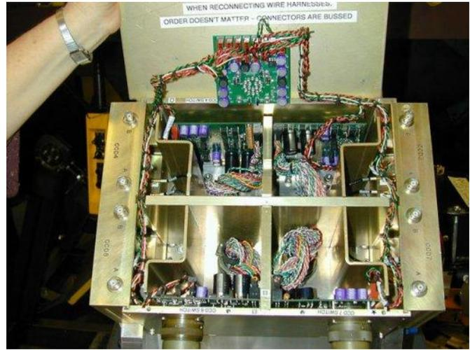
**Figure 5.** left, DEIMOS dewar with the science mosaic electronic boxes mounted on top; right, electronics box internals
