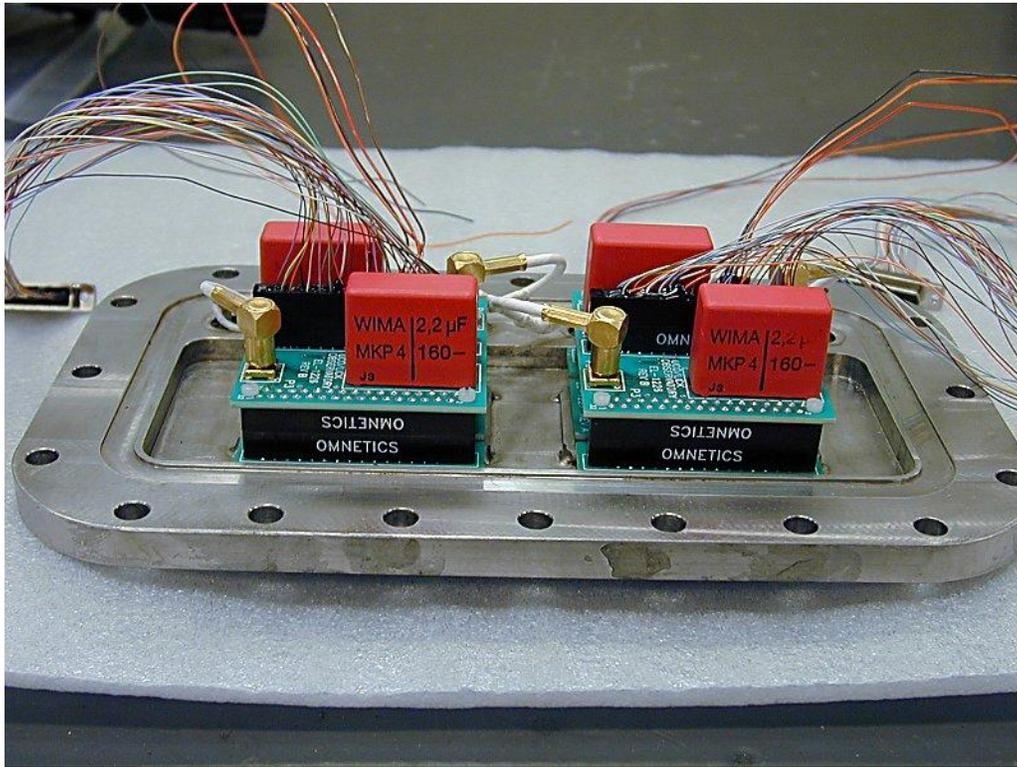
**Figure 6.** Earlier version of the detector vessel's FC plate indicating the internal circuit boards & CCD wiring harness. The harness is attached to the CCD Interconnect board, which piggy-backs onto the Hermetic Connector board.
