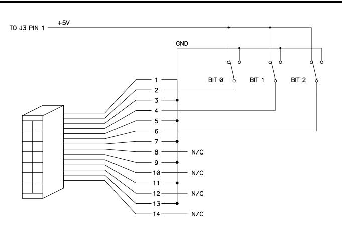
TO USE THIS TEST CONNECTOR, FIRST, REMOVE THE RIBBON CABLE CONNECTOR FROM THE ANALOG INPUT BOARD AND CONNECT THE TEST CONNECTOR. NEXT, REMOVE INPUT CONNECTOR J2 OR J3 AND INSERT THE RED WIRE INTO PIN 1. THIS CONNECTS +5V TO THE TEST CONNECTOR. NOW, SET THE BINARY WEIGHTED TEST SWITCHES TO SELECT ANY OF THE EIGHT ANALOG INPUTS. THE ANALOG VALUE CAN THEN BE READ VIA THE GALIL CONTROLLER OR WITH A OSCILLOSCOPE AT THE OUTPUT OF THE APPROPRIATE MULTIPLEXER CHIP.
