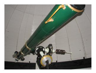
As many of these telescopes, this 13-inch was originally made by Dr. Henry Fitz in 1861, but the lens was reconditioned 11 years later by Alvan Clark due to a scratch across the lens. Today the telescope is "primarily used for the tour program and on occasion used to test instruments for the bigger telescopes" according to their website (http://www.pitt.edu/~aobsvtry/fitzclark.html). It is also used for astronomy classes.
