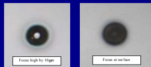
Example of a relatively large silver “spit” at two different microscope foci. The width of each image is about 40 \mu\text{m} . The appearance is roughly consistent with a hemisphere of metal (the bright central spot in the left image is actually an image of the light-filled microscope objective; the small spot just below and left of it is the image of a ceiling light).
