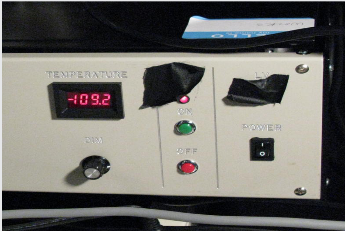
Figure 39. Power supply front panel meter showing CCD temperature.
