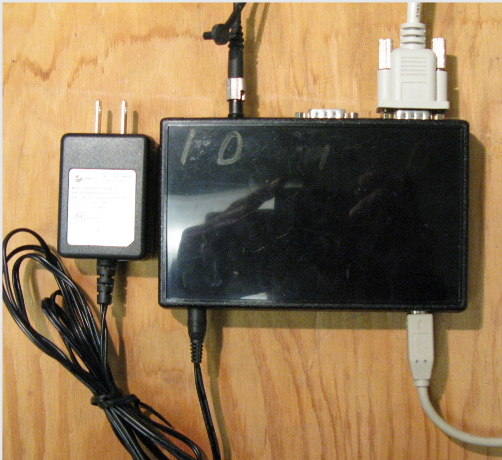
Figure 9. The UCAM USB interface is a stand-alone interface box.
