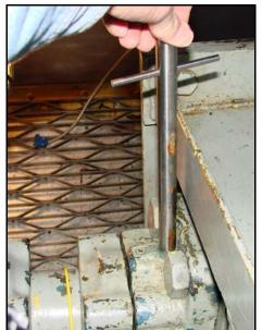
Adjusting tool ready to adjust the valve.
