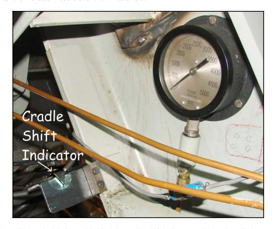
The alarm limit switch is located behind the cradle shift indicator and when installed years ago cclamps were used to temporarily hold the switch stops and are still there today.
