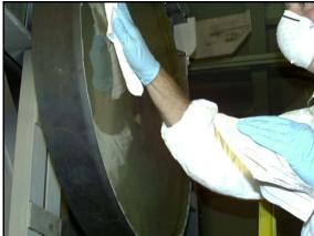
With the mirror in position, the surface is cleaned and dried with isopropyl alcohol and lint-free cloths (one soaked with alcohol, one for drying). Small segments at a time are worked, so as to not allow the alcohol to evaporate. It is important here to use high-intensity lights (as seen in the photo on the left, above), and view the surface at a glancing angle, which allows better viewing of dust and streaks.
