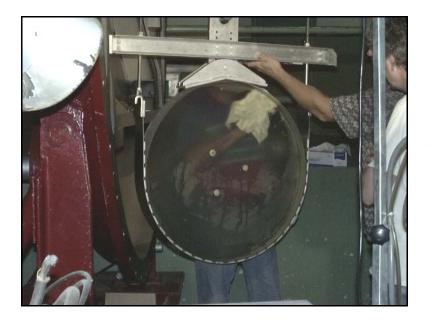
Once hanging from the hoist, the back side of the glass gets cleaned with isopropyl alcohol.
