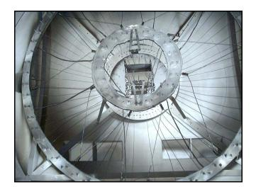
The business end of the coating chamber. This is where the filaments and the aluminum clips are mounted.
