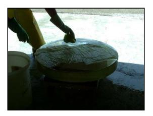
In areas where aluminum resists removal (this mirror is SIO overcoated, making stripping more difficult), a technique is to lay Kaydrys on the surface and saturate with stripping solution, and allow to remain for a time. Don't allow to dry, however.
