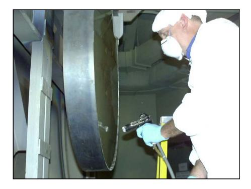
The final step is to blow off the surface with dry nitrogen through an anti-static gun, working from top to bottom. A final check of the surface is done, and if needed, spot cleaning with alcohol, and a blast with the nitrogen air gun. The chamber is then closed, and aluminization begins.
