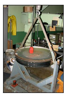
**Mirror Removal:** Use the dome crane and spreader bar to lift the secondary assembly off of the storage cage and roll the cage out of the way. Lower the secondary assembly down to a working height and leave suspended by the crane while removing the mirror. Remove two opposite side pads and attach the pivot posts. Now set the mirror and cell into the flipping frame.
