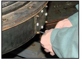
Remove the four bolts on the corners. Do not touch the setscrews with locking nuts. They are preset for positioning the glass properly.
