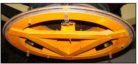
Bottom view of secondary frame with the mirror cell removed.
