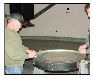
Remove the bolts holding the cell to the secondary frame and move the secondary frame out of the way.
