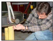
Set the mirror on the stool and remove the four safety clips and remove the cell.
