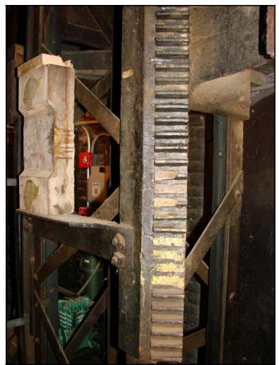
Here on this rack some upper teeth have broken out above the floor leveling section.
