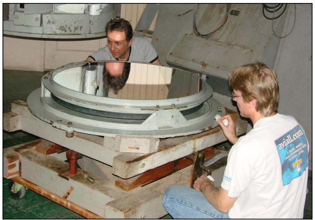
The finishing touches are done and the mirror is ready to remount in the telescope. Looks like a freshly coated optic.
