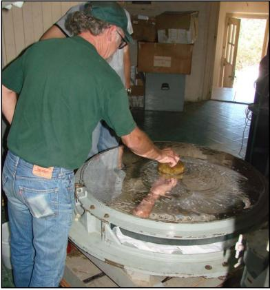
We washed the mirror in the cell using as little water as we could. The band for removing the mirror from the cell is missing so washing in the cell is necessary. Just be prepared for the water cleanup under and around the cell.
