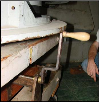
Make sure the mirror fixture is positioned so the crank clears the cell while lowering. We had to remount the cell and reposition the fixture.
