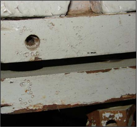
The mirror cell and mounting flange on the telescope are numbered for alignment purposes. This image shows position number three. There are a total of three mounting bolts to attach the cell.
