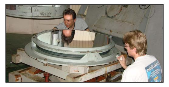
To start, install the RA support post. The top of the post has a rounded cutout that cradles the small weights on the end of the shaft. Use the wedge blocks to adjust the support height to level out the mirror cell and support the weight of the telescope once the mirror cell is removed.
