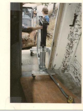
Install locking pins in Lixture to keep mirror from Swilleling, leave lifting fixture on.
