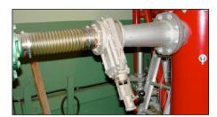
Open the valve located between the Roots blowar and cold trap. (left)
