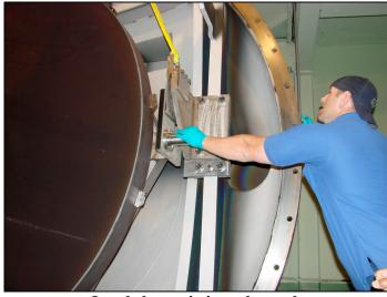
Load the optic into the tank
