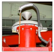
When the DP's are opened its time to fill the tank cold trap with liquid nitrogen. This trap is located on top of the DP valve chamber.
