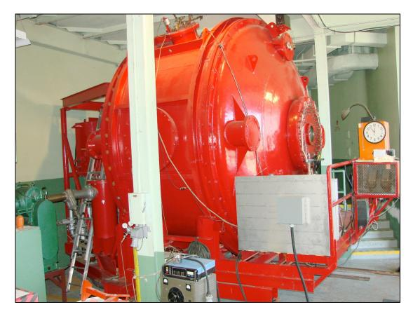
**Introduction:** This chamber is used for coating our Mountain optics. Our plans are to send most optics 40" and smaller to the coating chamber in Santa Cruz where they can do special coatings. We only coat with aluminum here and we no longer use SiO overcoating because of the light loss from this coating.
