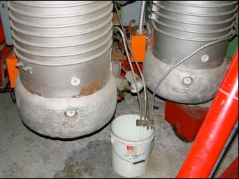
The hose from the sink goes to the Kinney pump. The valve on the wall to the right is the cooling water for the DP's. Open that valve fully. Watch that water is flowing into the bucket from all four cooling lines on the DP's. Run the black drain hose from the white pail to the floor drain in front of the coating chamber.
