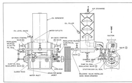
Fig. DVD 487 Diagram showing operating parts.
