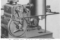
Fig. DVD 484 Lubricating Oil Seal Line to Closed Head.
