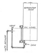
Fig. DVD 4811 Piping connection for automatic drainage of moisture from separator.
