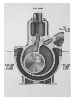
Fig. DVD 485 Rotating Plunger rapidly creates space for gas in pump chamber.
