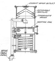
Fig. DVD 489 Oil Separator, steam heated.
