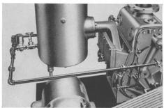
Fig. DVD 483 Lubricating Oil Seal Line to Open Head and Stuffing Box.
