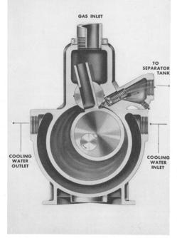
Fig. DVD 486 Rotating Plunger approaching end of discharge expels gas from chamber.
