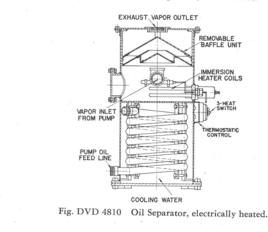
In operation, oil discharged from the pump into the upper chamber falls on the heating coil where water is flashed off. All oil collected in the upper chamber then flows through the by-pass from the upper chamber into the cooling coil immersed in water where it is brought to proper temperature before returning to the pump. Vapor flashed off by the heating unit rises and
