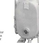
RIGHT - Sight Glass for Oil Level Indication in Gearhouse of Booster
