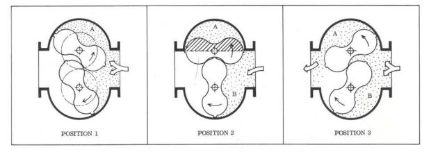
Impeller Rotation and Gas Flow through a Vertical Roots Pump
