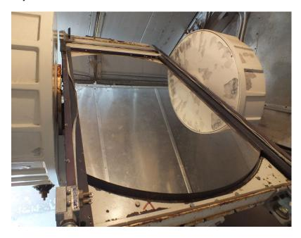
The next CAT mirror, M2, faced downwards at a 45 degree angle, so it wasn't too dirty. Dave cleaned it and we measured 83% with the blue filter and 88% with the red. There is some severe paint chipping from the housing that can be seen in the photo; it could and probably does fall down from that level to the primary mirror below.
