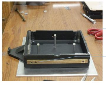
Grating removal jig and cell after grating was removed
