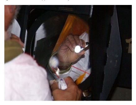
The prism access was open, so Dave wiped it with ethanol. That streaked, so he wiped it again with acetone. In this photo he blows the dust off the grating.
