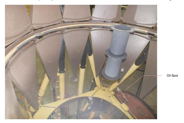
**CAT Primary**The Coude Auxiliary telescope's up-facing primary is almost always dusty, and this trip was no exception. Dave cleaned it with sprayed on de-ionized water, followed by ethanol or acetone.
