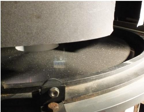
**Dome Samples**Here are some pictures of the upward-facing 2" Zerodur disks undergoing long-term environmental testing in the dome. The downward-facing ones were not photographed because, without removing the rack the angle makes it difficult to get a decent shot.
