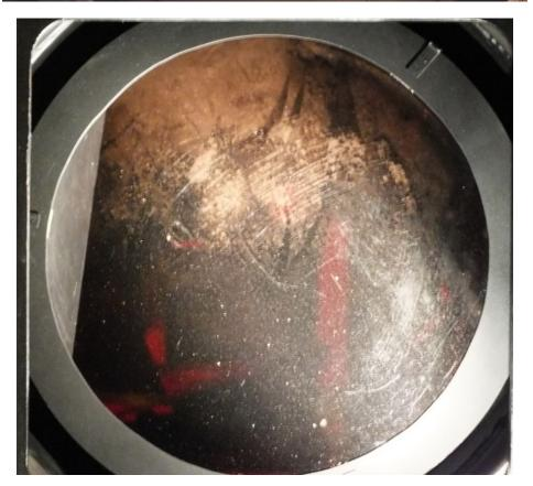
Dave blew the optic off with canned air but decided the coating was too fragile to safely clean. What was surprising was that the bottom part of the optic didn't look too bad, considering we had seen what looked like degradation on a previous trip. It turns out the optic with the degradation on the bottom was a different mirror that had been positioned in front of the Hamilton Collimator at that time (August).
