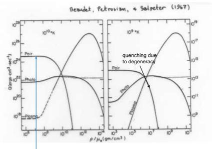
note that units here are erg cm<sup>-3</sup> s<sup>-1</sup> not erg g<sup>-1</sup> s<sup>-1</sup> Per unit volume pair rate is roughly independent of density until degeneracy cuts it off.
