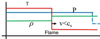
A detonation is a supersonic burning front in which a shock wave heats and compresses matter causing it to burn. If the rise in pressure from burning is large and rapid enough it drives the shock wave and keeps it from decaying. Pressure, density and temperature all rise in a detonation
